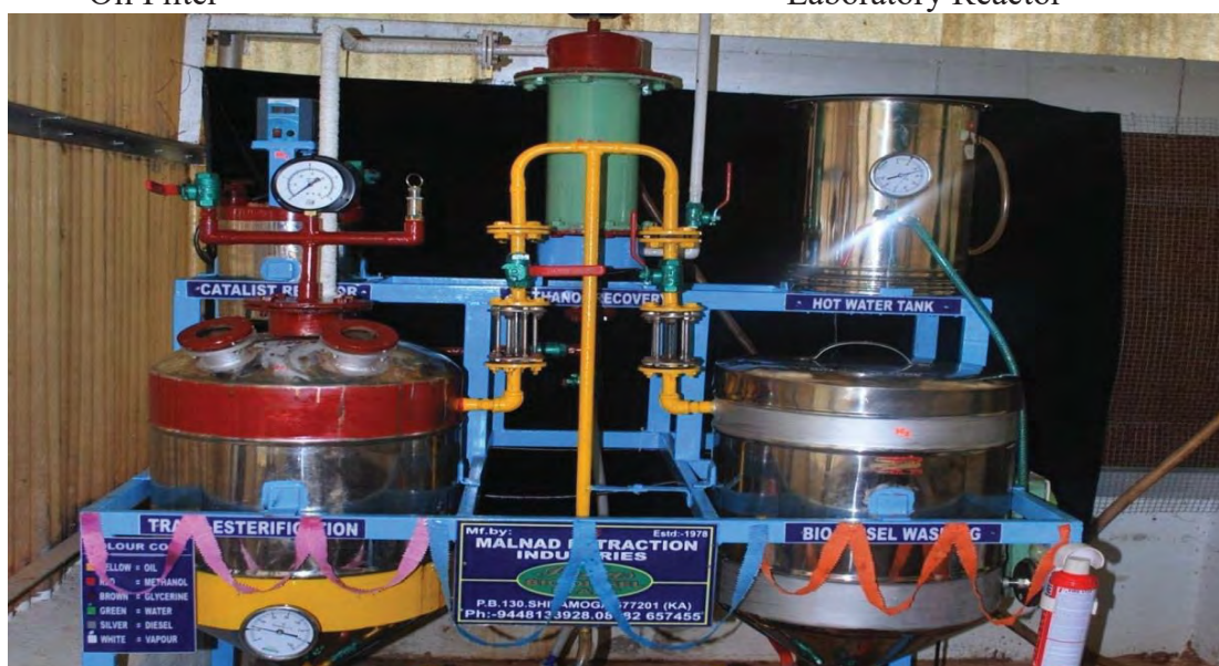
A simple low cost stainless steel body 50 litre per batch Esterification unit.
